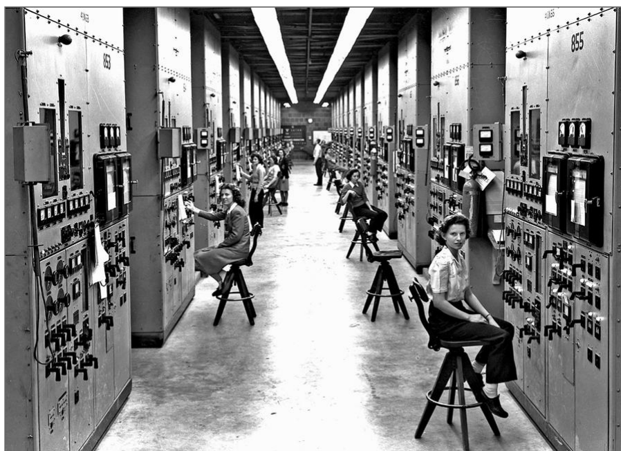
6. Calutron operators at their panels, in the Y-12 plant at Oak Ridge, Tennessee, during World War II. The calutrons were used to refine uranium ore into fissile Read more +
